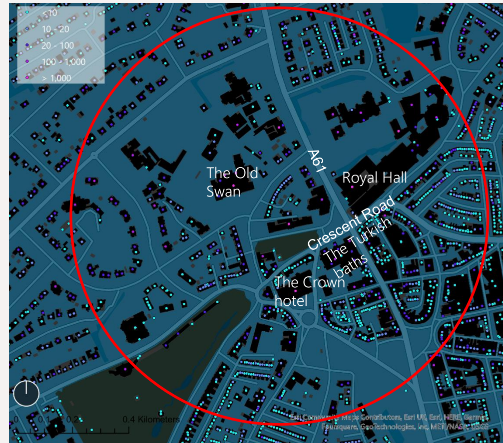
Heat demand for buildings in Area 1 of Harrogate heat network starting points (MWh/year)
