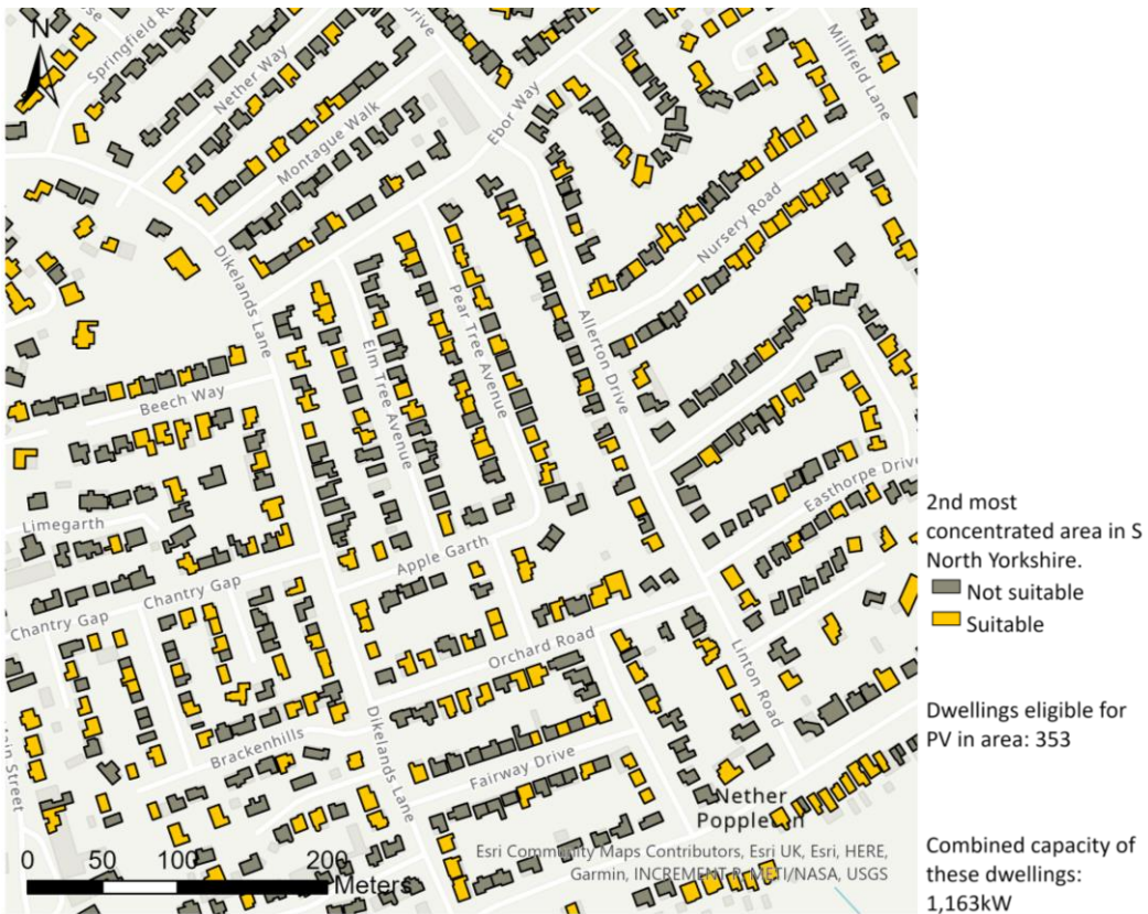
Figure 61: Dwellings identified as suitable for rooftop PV panels. (Location: Nether Poppleton, York )
