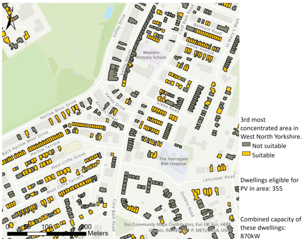
Figure 95: Dwellings identified as suitable for rooftop PV panels. (Location: Central Harrogate )
