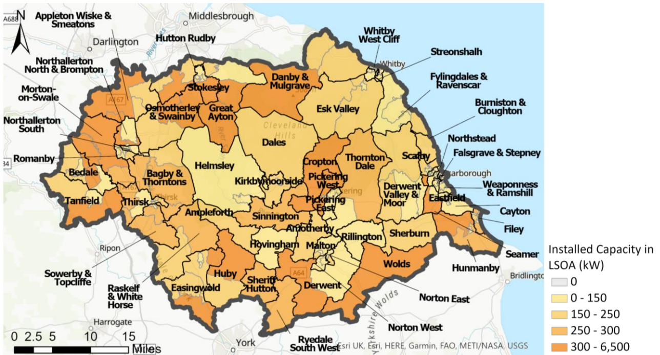
Figure 25: Aggregated capacity of renewable installations registered for FIT within each LSOA of the East North Yorkshire sub-region.
